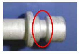
7. Install the O-ring (Small) of the O-ring kit to the A/C pipe (HI).
