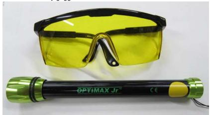
3. Direct a black light toward the joint part between the expansion valve and the A/C pipes (HI and LO) and look for a refrigerant leak.
